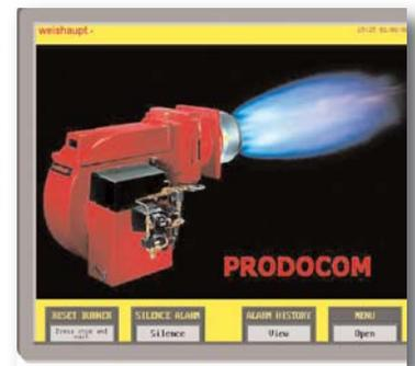
**The Bottom Line:** The first month of operation yielding 586 hours of operation with a mere 49 cycles. The burners were turned at 10:1 turn-down with O<sub>2</sub> levels at 3%.
